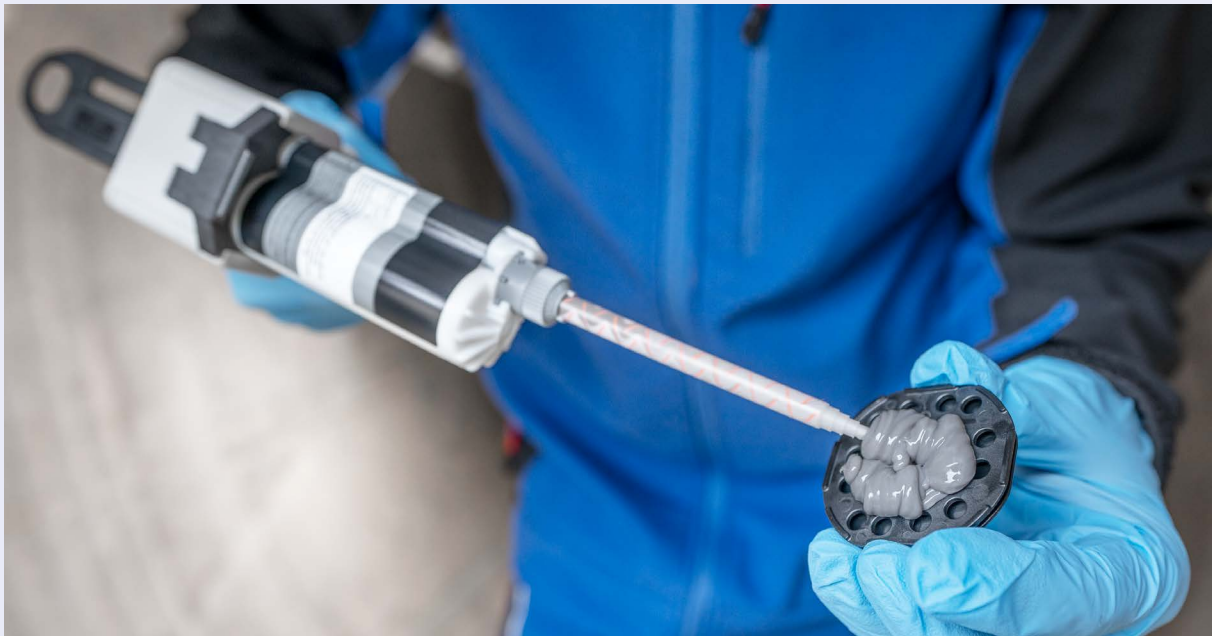
Use the application tool to apply 3 spots of adhesive in a pile on the surface to be bonded.
